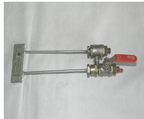
Fig 3 Flat-Jack used for test
