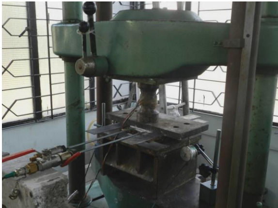
Fig. 4 Arrangement of calibration test
